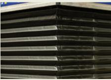
Protective bellows mounted on a lift table
